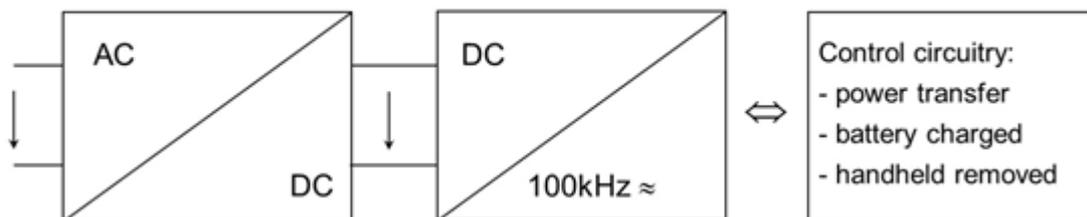
*Scheme: Optionally a DC source of 4 – 32 V can be used, depending on the transmitted power.*
