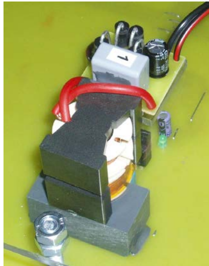
„Pick Up Core“ for a secondary unit.
