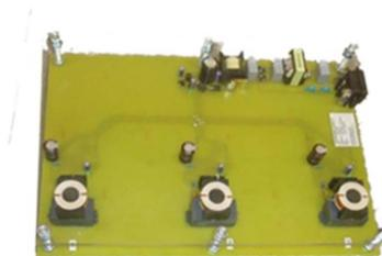
*Example: Inductive or contactless charging respectively for up to 3 appliances*
