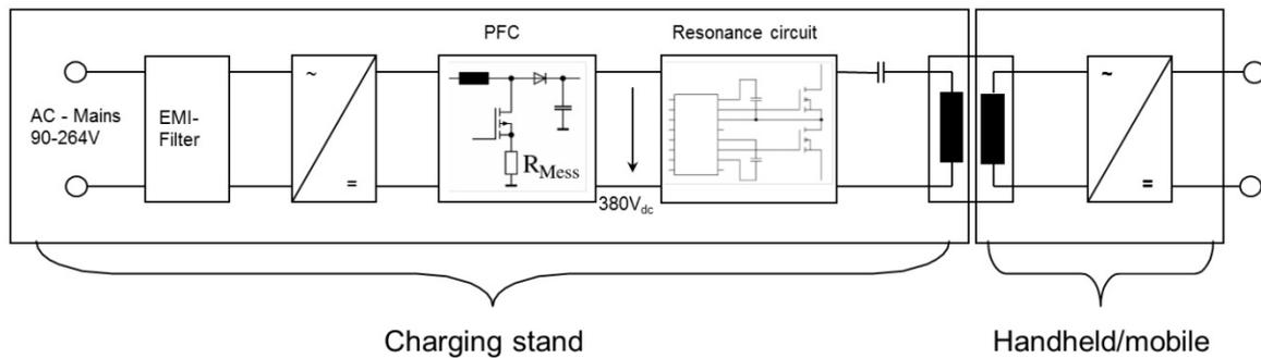
*2-stage approach: PFC as 1st stage, offers sinusoidal input current in accordance with EN61000-3-2*
