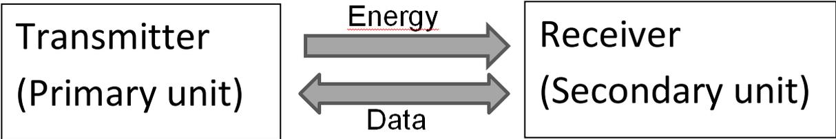
Scheme : Energy transfer from primary unit (transmitter) towards secondary unit (receiver). Data transfer in both directions with up to 500 kbit/sec
